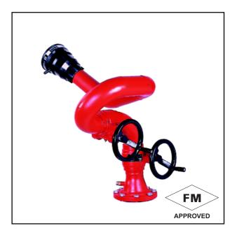
resistance. The vertical and horizontal rotation is through corrosion resistant bronze swiveling joints with double row of stainless steel ball bearing. Both vertical and horizontal movements are controlled with hand wheel driven fully enclosed worm gears and protected from the elements.
